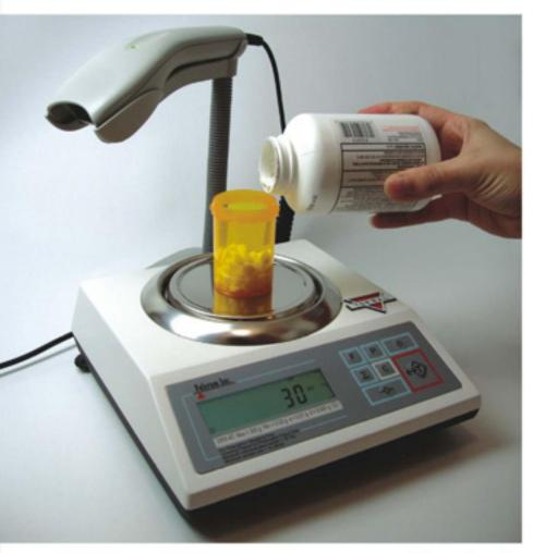
The DRX-4C is equipped with an NTEP-approved, legal-for-trade counting feature for prescription filling. The scale counts up to 90 pills per second with a database capacity that allows it to store over 3000 NDC codes and pill weights. New drugs and their NDC codes are quickly and easily added to the database, which may be maintained by updating the stored sample sizes and weights.\* The
